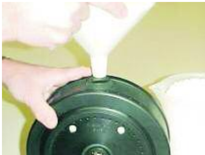
Figure 6 a, Refilling Soda Lime
